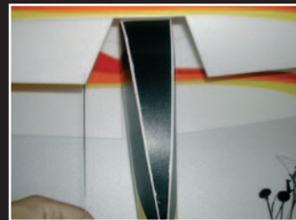
Link upper ailerons and lower ailerons together using the in-between aileron links.
