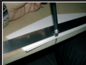
Prepare the elevator making a 60° angle at the trailing edge edge.
