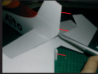
Make slots in the fin for the hinges.
