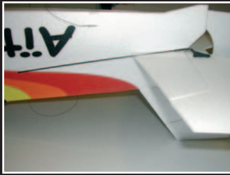
Installing the elevator link to the elevator.
