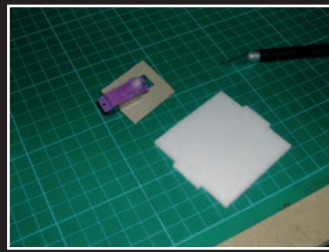
Locate the plate for the rudder servo.
