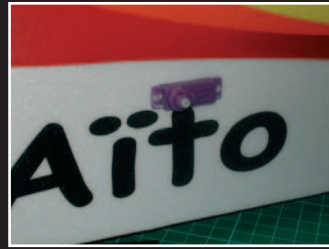
The servo is still glued in place. Use enamelled wire for extensions. This will save you at least 7g on the total weight.
