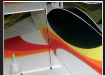
Link upper ailerons and lower ailerons together using the in-between aileron links.
