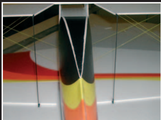
in-between aileron links in place.
