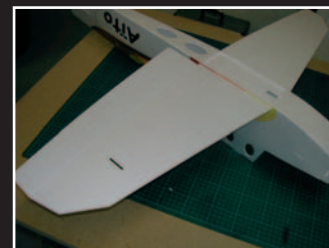
Insert the lower wing into the fuselage.
