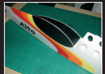
Gluing the canopy's top in three steps. Use activator for easier work.
