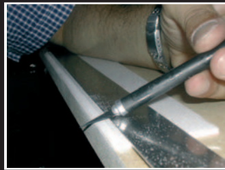
Prepare the ailerons making a 60° angle at the leading edge.
