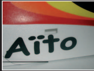
Make hole for the elevator servo.
