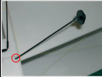
Positioning the landing gear legs. Glue on the red points.
