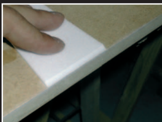
Sand the trailing edge of the canopy's top at 45°
