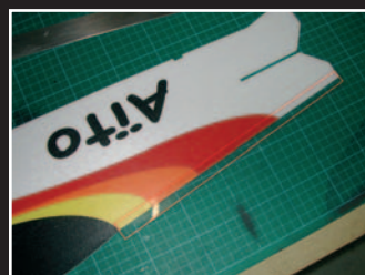
Apply hinge tape on the outside dorsal edge of one fuselage side.
