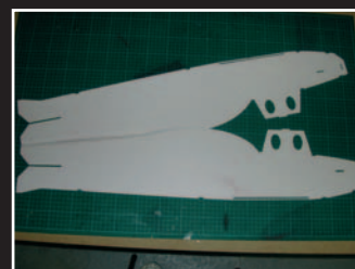
Join the two fuselage sides with hinge tape already in place on the other side.
