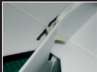
Installing the rudder horn. Please insert the horn through the lower hinge.
