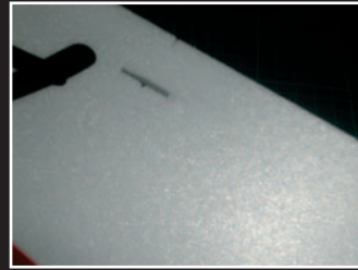
Cut off a small rectangle at the back of the fuselage on both sides. These rectangles are made for the passage of the rudder wires.
