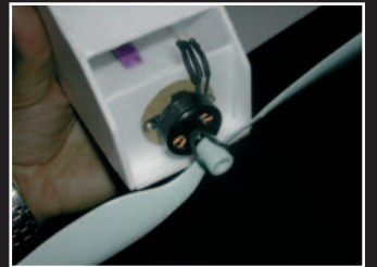
Installing your motor. You may use the smaller plate and the 1mm PVC Plate. Once your motor is fixed, insert the plate into the fuselage sides holes.
