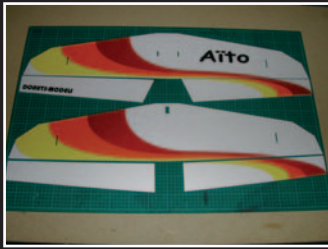
Prepare the wing by cutting the ailerons from the wings.
