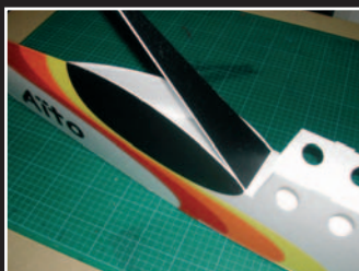
Gluing the canopy's top in three steps. Use activator for easier work.
