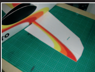
Drill the opening for the landing gear legs. 50mm above the leading edge of the lower wing.
