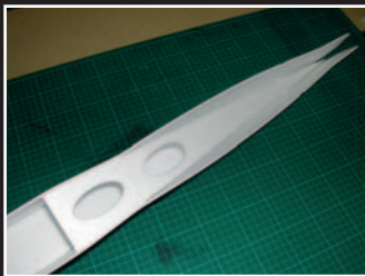
Place and glue the smaller horizontal piece between the two lower fuselage sides.
