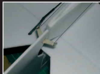
Link the wires to the rudder horns. Tension the wire.
