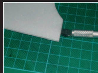
Make the slots in the hinges for the rudder.
