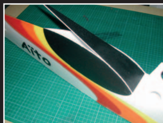
Gluing the canopy's top in three steps. Use activator for easier work.
